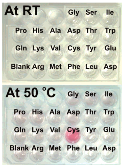
Figure 2. The colorimetric response of the DNA–Au NP/Hg 2+ complex aggregates in the presence of the various amino acids (each at 1 \mu M) at room temperature and 50 ^{\circ} C.
